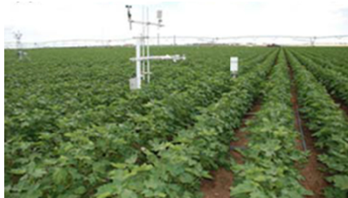
Figure 2. Cotton field with instrumentation installed above the lysimeter box, at the USDA ARS CPRL, Bushland, Texas, USA
