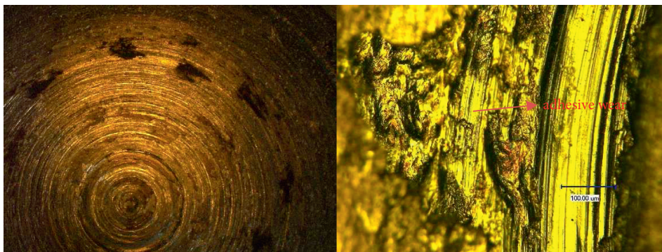
FIGURE 13: Dry grinding morphology diagram of the optimal orthogonal sample group.
