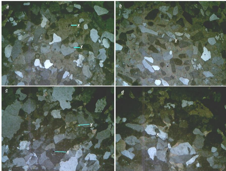
Fig. 6a-d. Photomicrograph of studied samples taken under cross polarized light illustrating subangular to subrounded poorly sorted grains and porosity types. (x – intragranular; y - intergranular).
