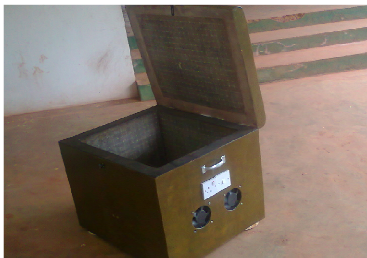
Fig. 4. Locally designed and fabricated acoustic enclosure for mini generators
