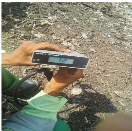
Fig. 3. Measurement of oxygen % by OT meter
