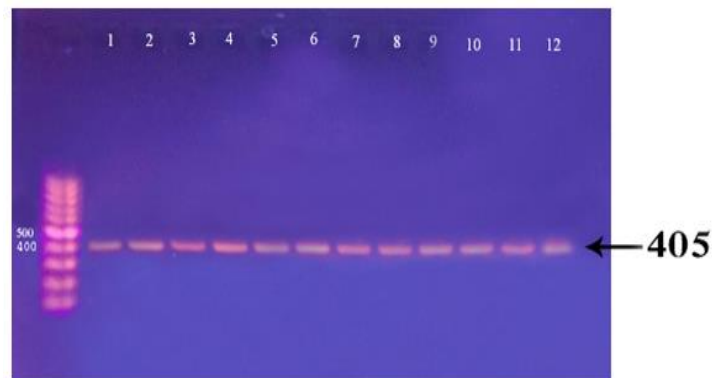
Fig. 3. 1% after staining with ethidium bromide, erna PCR products were electrophoretically separated on an agarose gel at 70 volts for 50 minutes and visualized under UV light at 301 nm. L: 1500 bp ladder; lane (1-12) was positive for this gene; the product size is 405 bp
