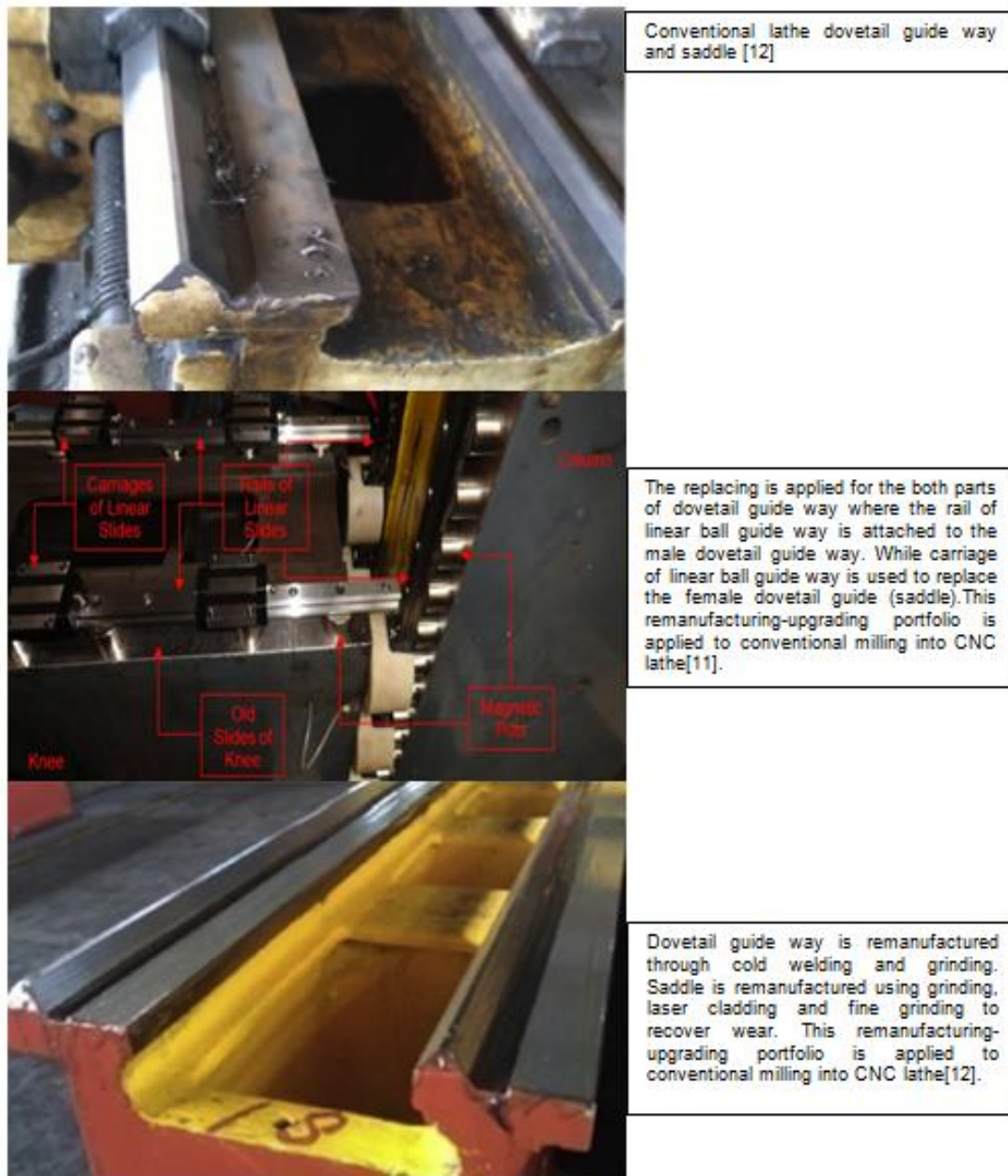
Fig. 10. Insert/mate/screw ball linear guide based assembly and dovetail guide way based remanufactured [11][12]
